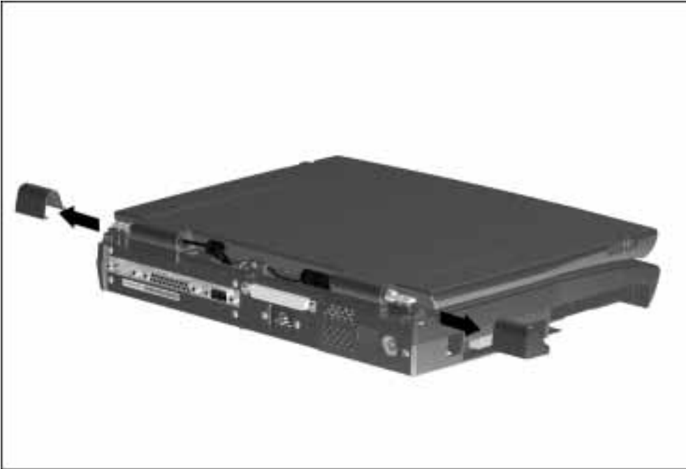
Figure 7-22. Removing the Clutch Covers
