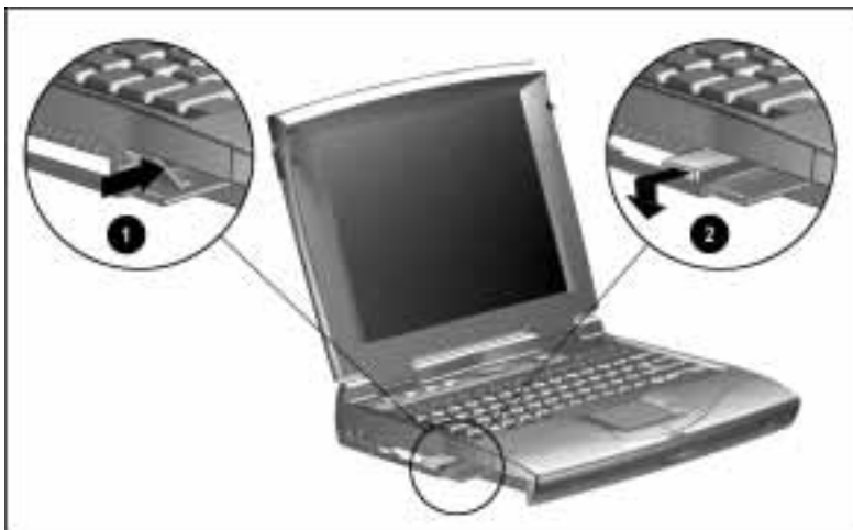
Figure 1-1. New Battery Spacer Door
