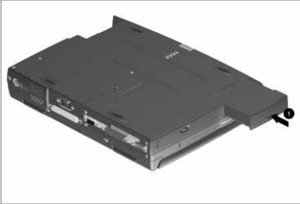
Figure 7-3. Inserting the Battery Pack
