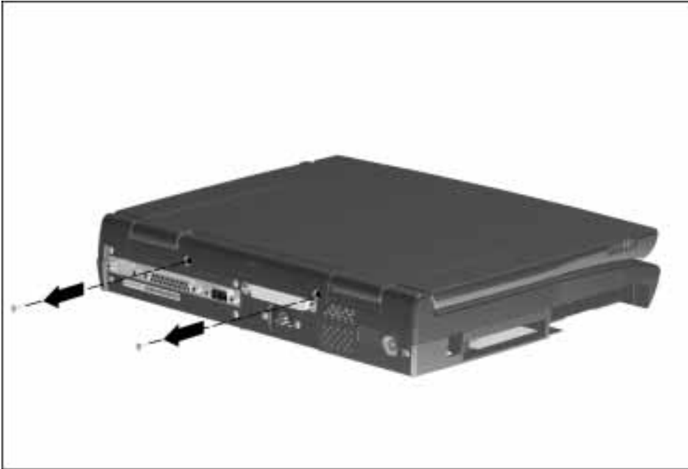
Figure 7-19. Removing the Microphone/Display Cable Cover Screws
