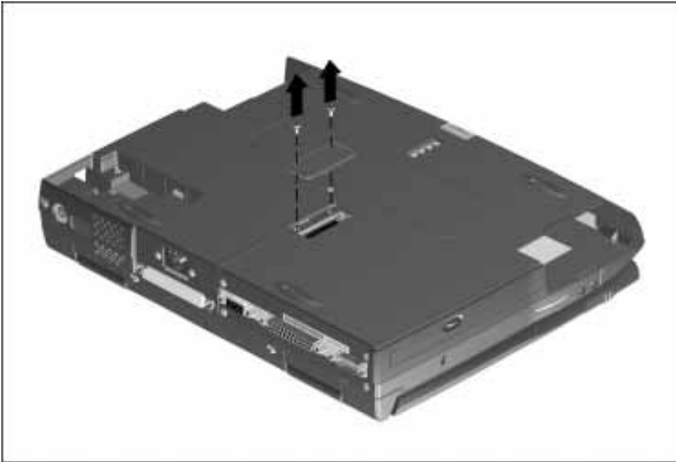
Figure 7-7. Removing the CD-ROM Drive Access Door
