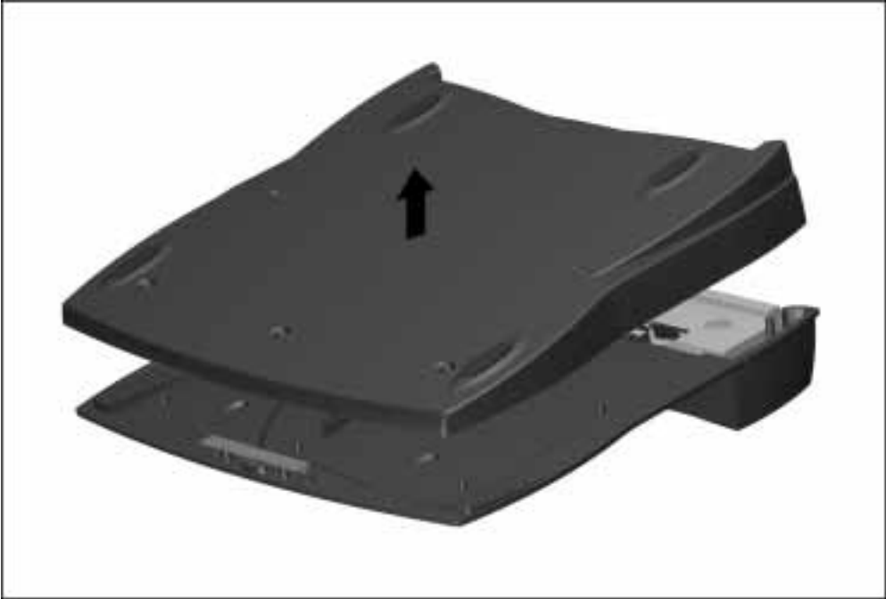
Figure 8-2. Removing the Base Plastic Housing
