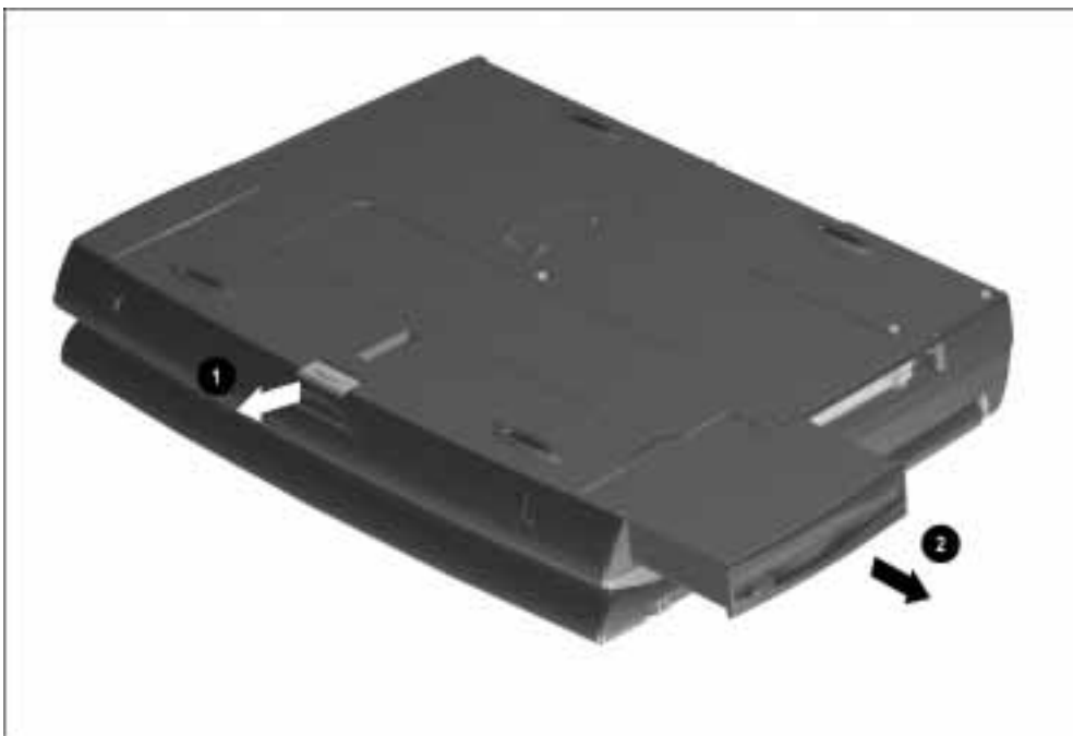
Figure 7-4. Removing the DualBay Device
